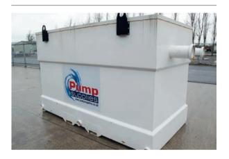
Our fleet contains a varied range of settlement tanks for use on the pump discharge, which are specially designed to prevent silt and fines being discharged into the water course or drains. Each tank has a series of weir plates to slow the flow of water allowing settlement; they are also fitted with Bauer couplings to suit any application, lifting eyes and drain plugs for cleaning.
