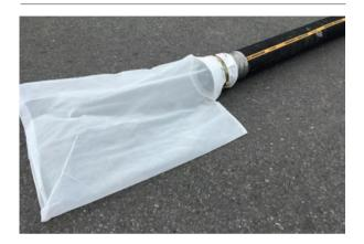
We have available from stock 100 micron to 250 micron silt bags or fabric filters (other sizes are available). In addition to settlement tanks they are a very effective way of helping solve the ongoing environmental issue of removing suspended solids from water on civil engineering construction sites. Silt bags are easy to install and are generally found at the end of the discharge line where silt removal can be monitored and inspected.
